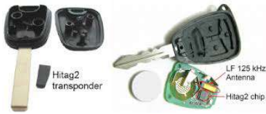
Fig. 1: Car keys with Hitag2 transponders shown in [11]
